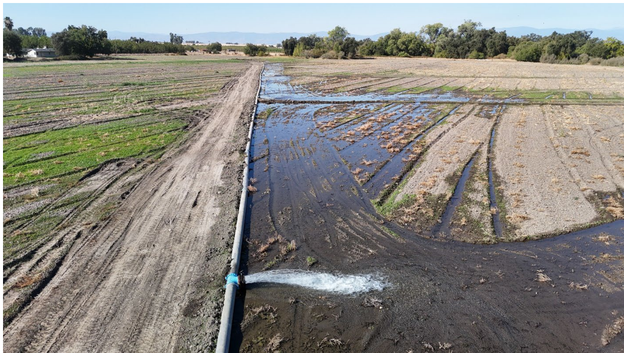
Figure 3-2. Pilot Test #2 Basin Showing Pipeline and Outlets
