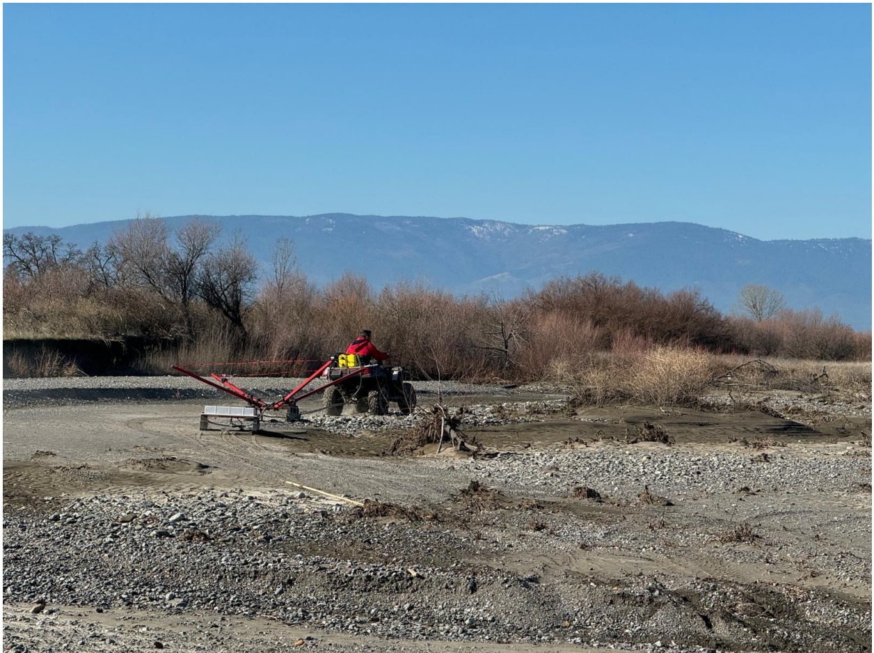
Figure 3 The transmitter loop (red wire) attached to a frame with red arms that is mounted on a sled (black). Similarly, the receiver coil (white box) is mounted on a sled and pulled behind the transmitter loop.
