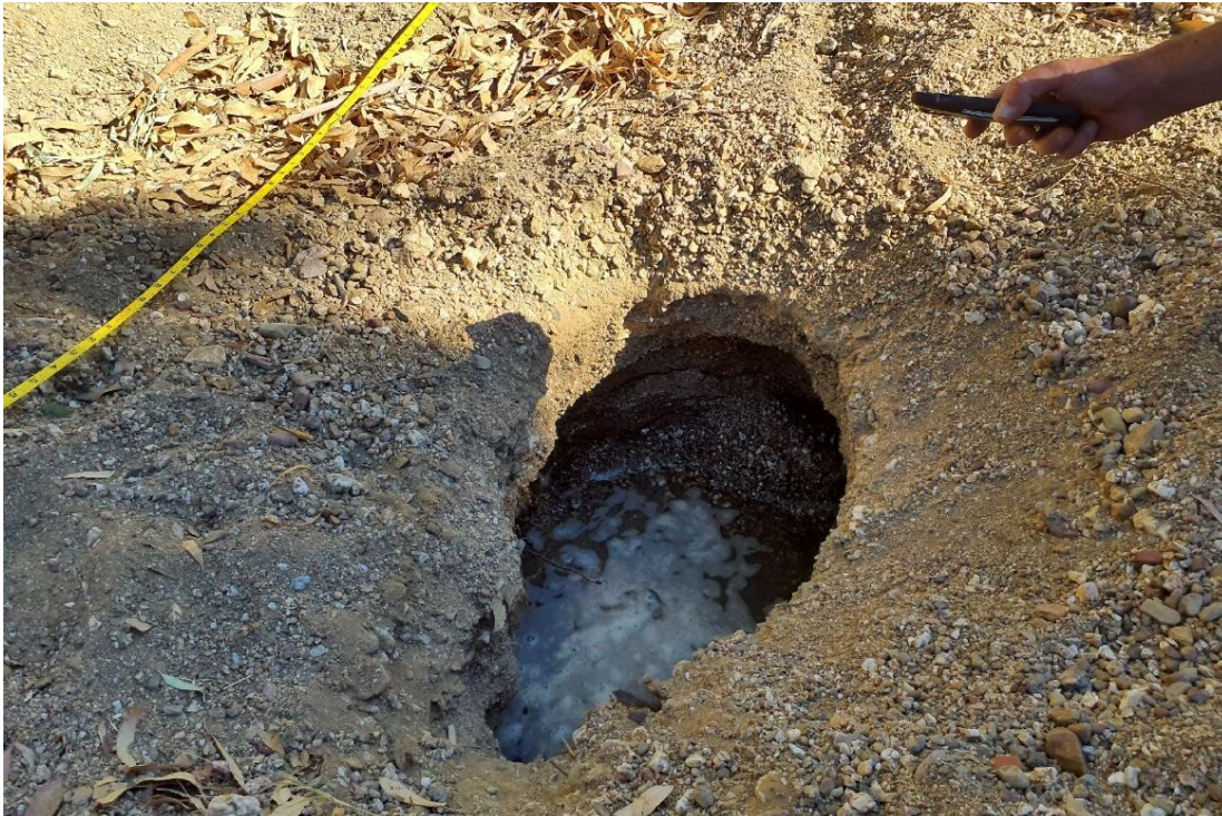
Figure 7. One of three holes excavated to investigate the existence and depth of a potential confining layer beneath the Brannin Creek streambed. Standing water at a depth of 1.5 FT below the surface was observed at this and the other two test holes.
