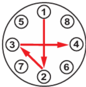
Suggested Tightening Sequence
