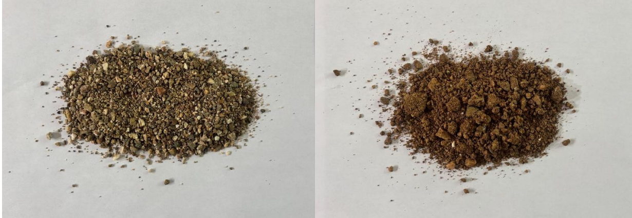
Figure 8. Soil samples retrieved from Brannin Creek Streambed, showing the soil above the confining layer comprised of sands and gravels (left), and soil within the confining layer (right) comprised of smaller particles that bind together into a hardened material.
