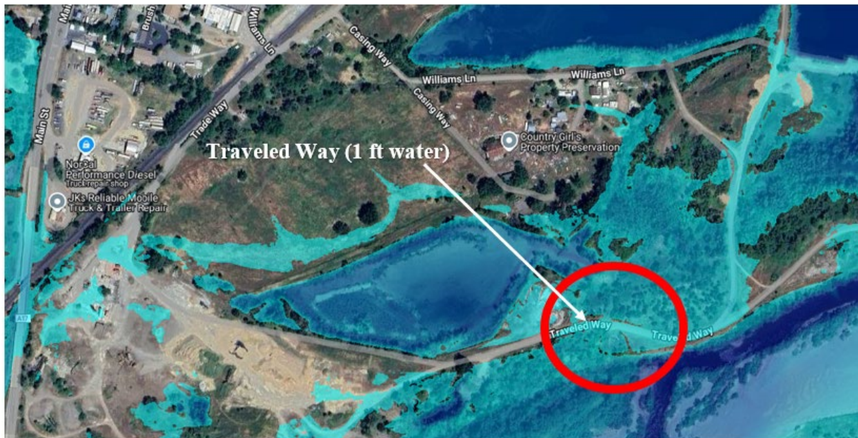
Figure 28. Traveled Way Impacted at a 10-Year event.
