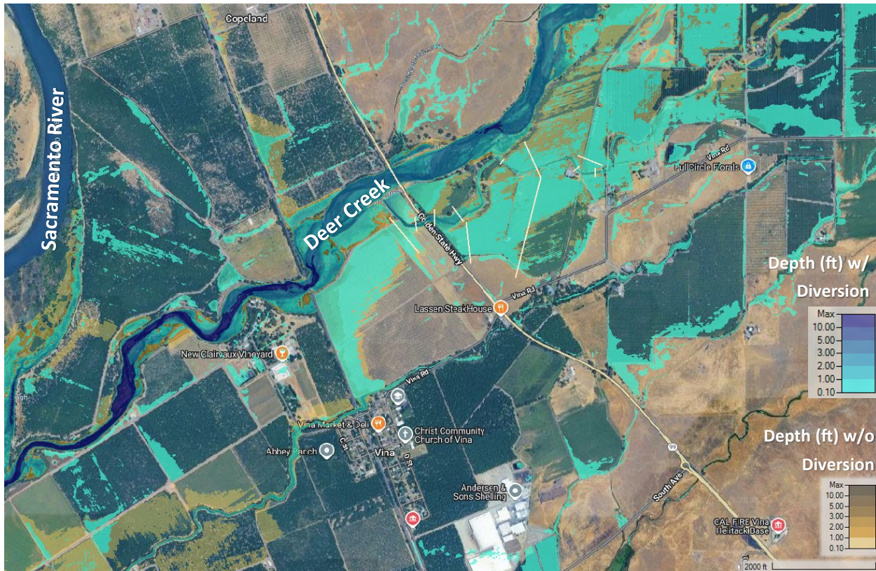
Figure 12. Maximum Inundation Area Comparison between Original Scenario (brown) and Diversion Scenario (blue) for the 50-Year Event in the Lower Deer Creek below USGS Gage 11383500
