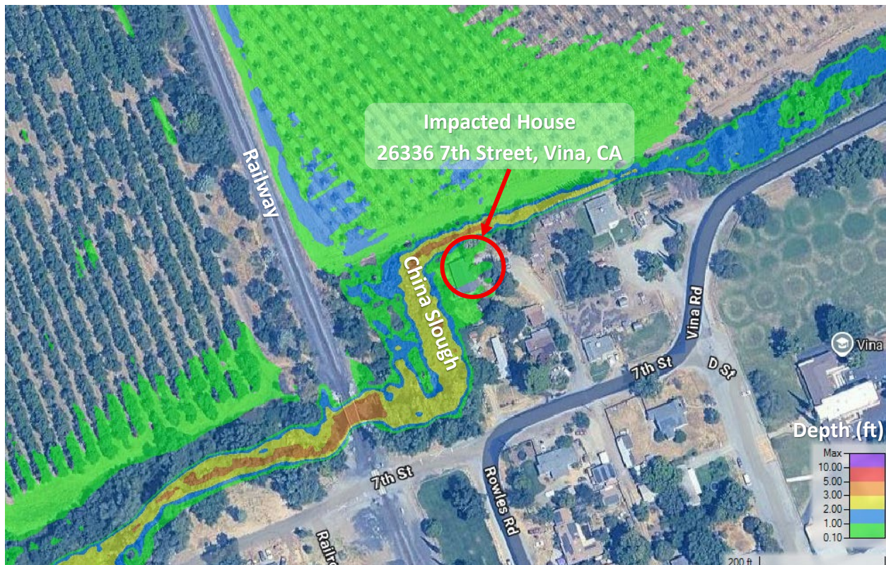
Figure 8. Inundation Map of the Residential Area in Vina, CA during the February 2025 Event
