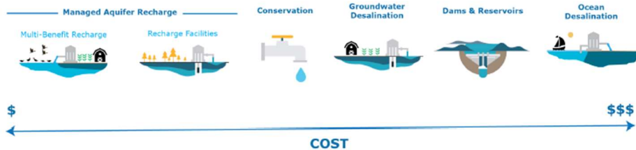
Figure 4. Water supply cost comparison, with the cost per unit of water increasing left to right.
