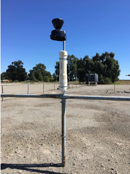
Figure 14. Rain gauge installed at Program site.
