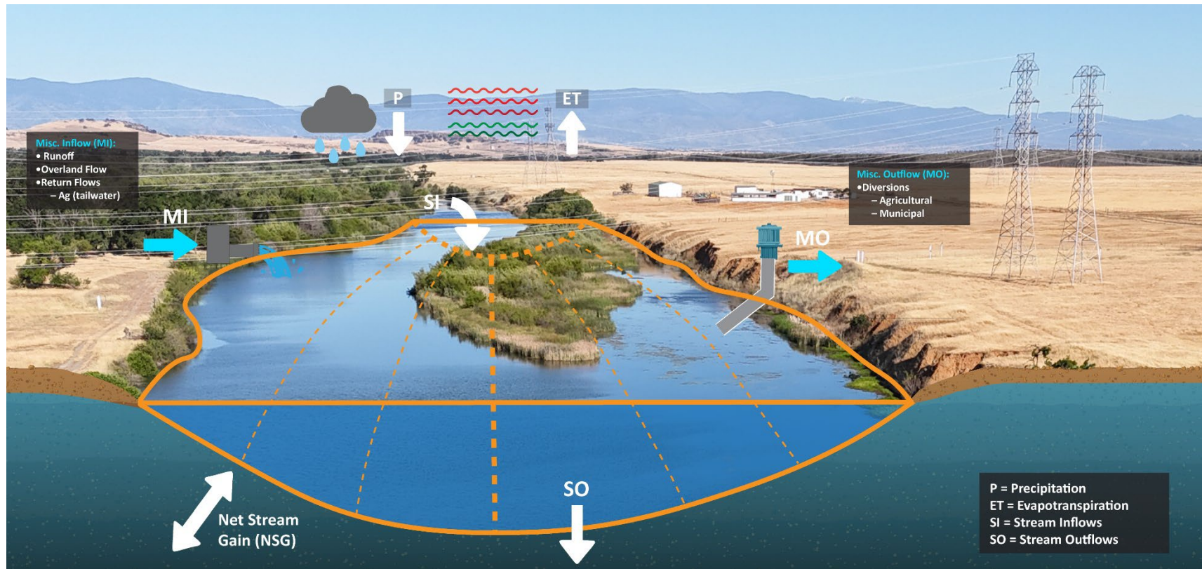
Figure 4. Conceptual illustration of a stream reach water budget for Stony Creek in Tehama County showing the major flux components used in the Study. Stream inflows (SI), stream outflows (SO), precipitation (P), evapotranspiration (ET), miscellaneous inflows (MI), and miscellaneous outflows (MO), and net stream gain (NSG) all contribute to the stream reach water budget for a defined reach (outlined in orange). This framework allows field measurements and estimated fluxes to be integrated to quantify NSG and evaluate stream–aquifer interactions. Note that stream outflow (SO) is the amount of flow continuing downstream of the stream reach in the surface stream even though the arrow could be misinterpreted to mean that it is infiltrating through the streambed. A stream reach water budget schematic is also included in Figure 7.
