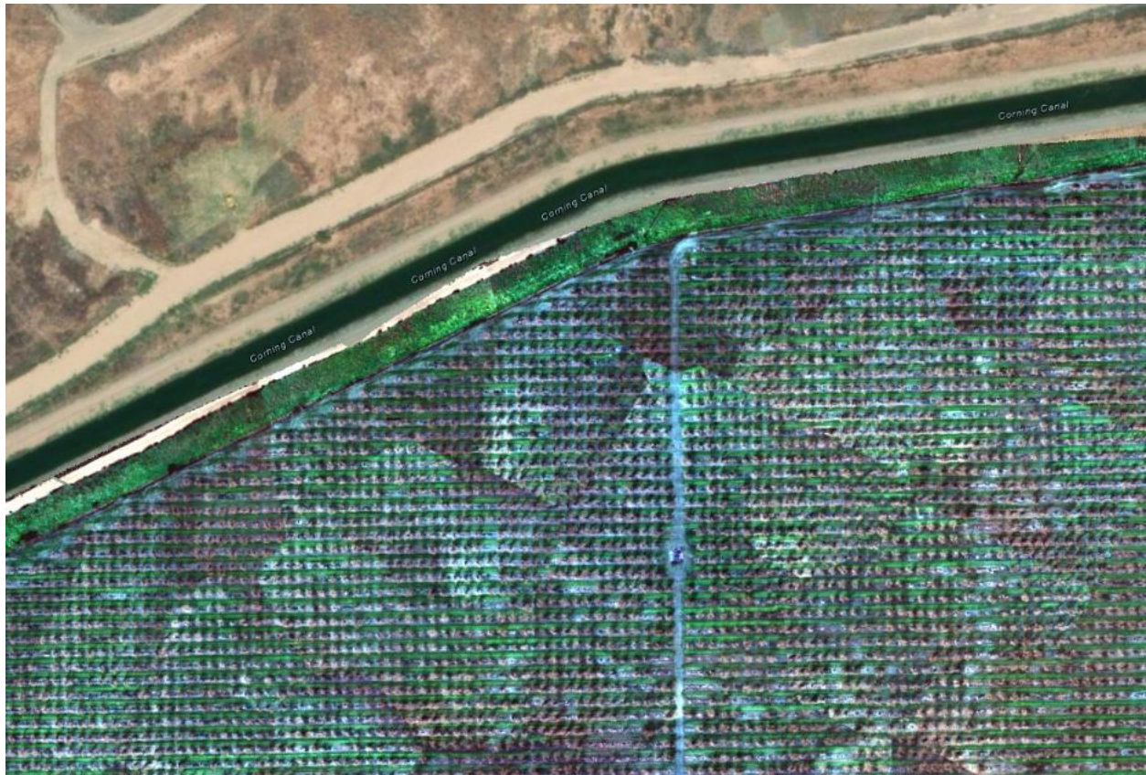
Figure 2. Example multispectral scan from a field within Lindauer River Ranch. Bright green coloration indicates chlorophyll levels to determine vegetation health.
